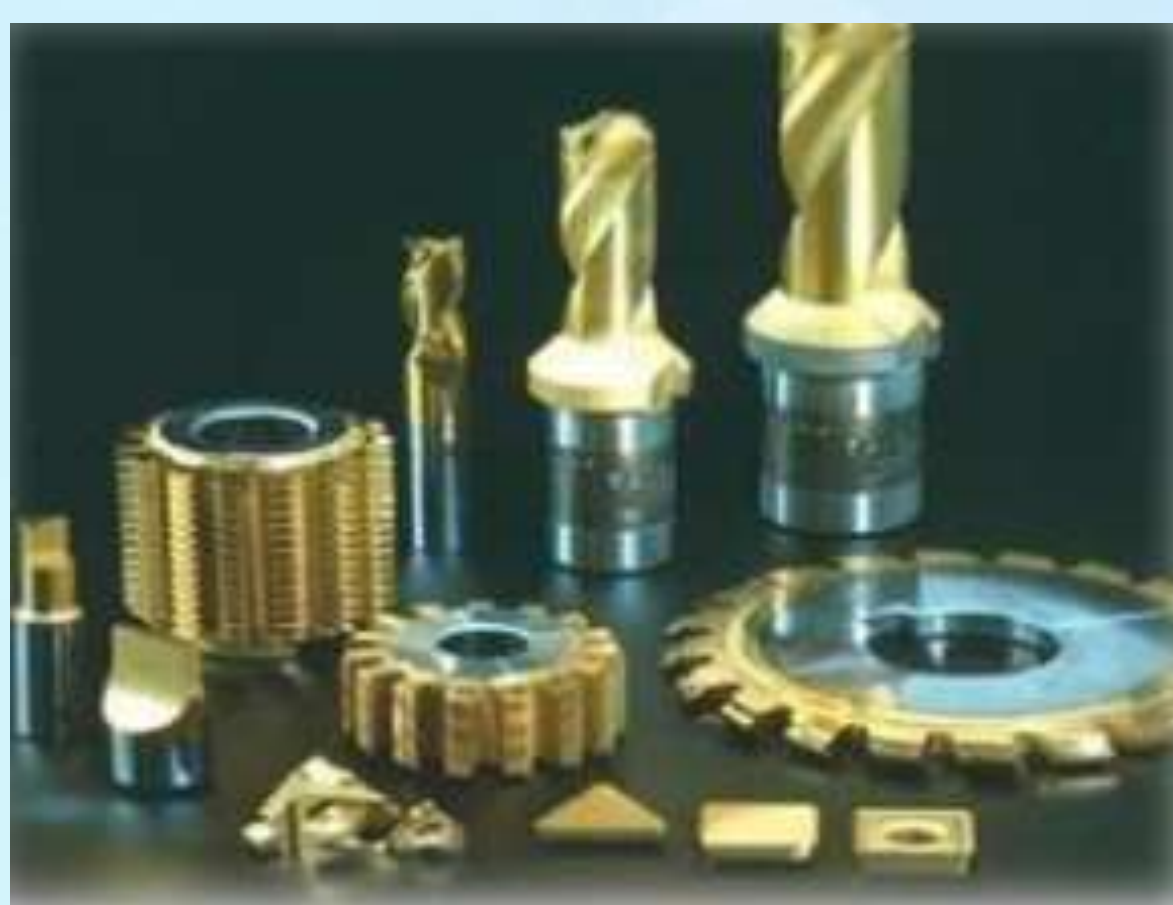
Hard Coatings on Cutting Tools
